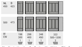
NL = Nominal length D = Depth W = Width CW = Carcase width
